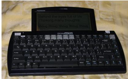
Fig 3.1 Keyboard text-to-speech generating device<sup>25</sup>
